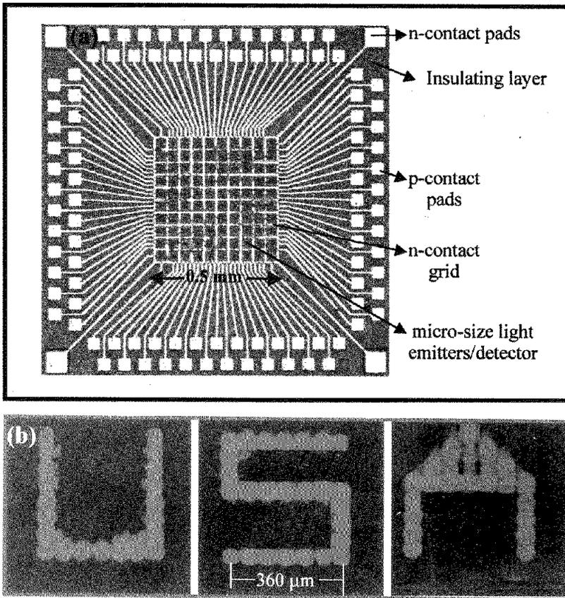
Figure 3. Optical microscope images of (a) a bonding scheme that allows us to address each microdisk pixel individually (or a III-nitride blue microdisplay); (b) the III-nitride blue microdisplay (a) in action.
