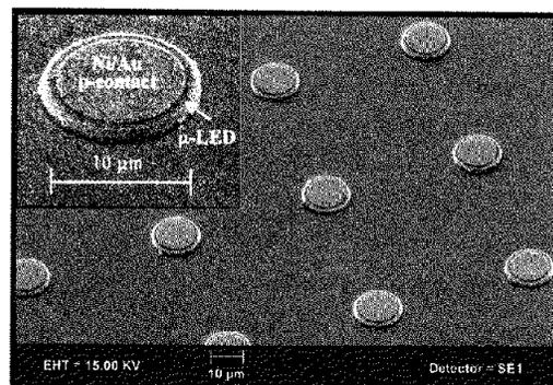
Figure 1. Scanning electron microscope (SEM) image of a III-nitride micro-size LED array.
